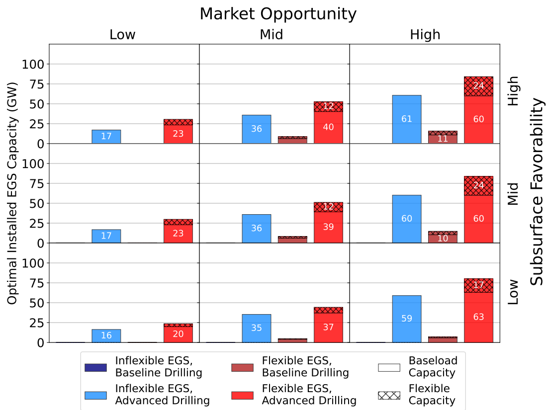
Supplementary Figure 4: EGS deployment potential in 80% decarbonized electricity systems. Same as Figure 2 in the main paper, for scenarios with a 80% clean electricity requirement. Data labels are provided for capacities greater than 10 GW.
