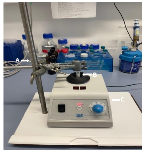
Figure 7: Improvised agitation device. Bead tube containing sample (B) held by the retort stand (A) on top of a vortex (C) at 2,400 rpm speed for 12 minutes for cell disruption of Gram-positive V. salmoninarum cells.
