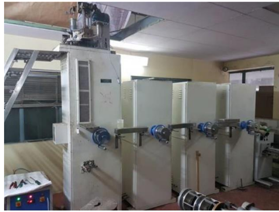
Figure 2: The pilot melt spinning machine used to develop filaments yarns
