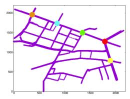
Fig. 3: Reference scenario: road topology in the city of Bologna. Circles represent RSU locations. Distances are expressed in meters.
