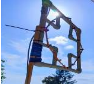
Fig.2 b). Loop antenna – real life model.
