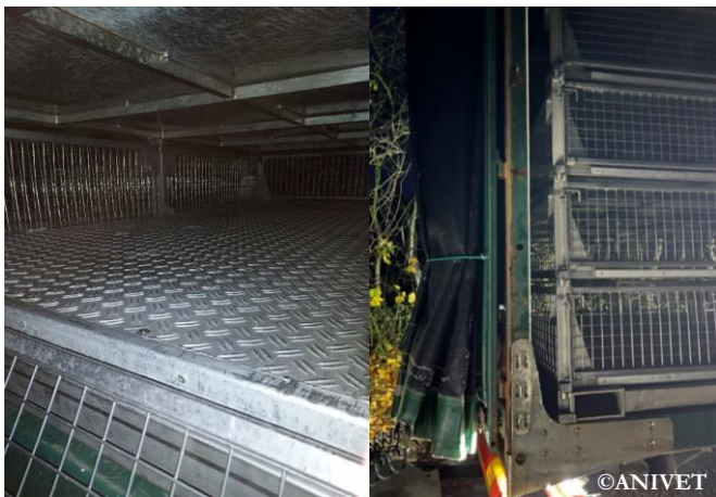
Left: the floor in the containers; Right: the curtains in the storage position
