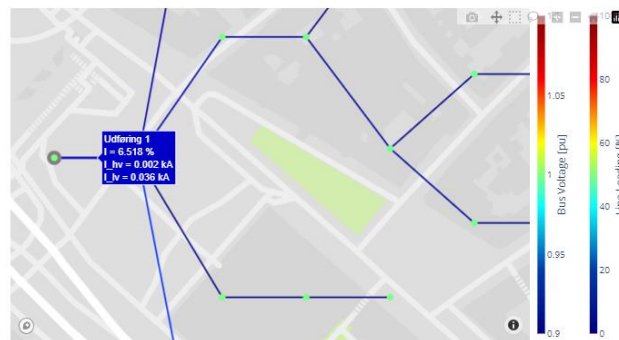
Figure 43: Transformer loading in blue color
