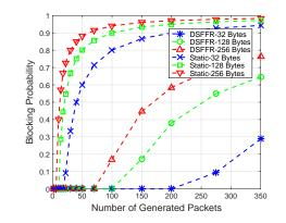
Fig. 3: Blocking probability comparison between DSFFR and static case for  $\alpha = 2.1$ .
