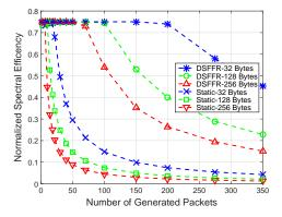
Fig. 6: Normalized spectral efficiency of DSFFR compared with the static case for  $\alpha = 4$ .
