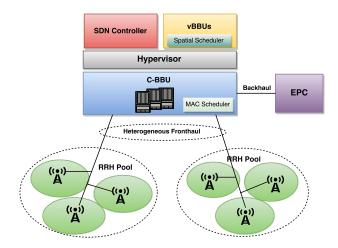
Fig. 1: C-RAN system architecture including SDN control and NFV.
