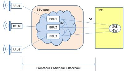
Figure 1 – Xhaul general architecture for 5G networks
