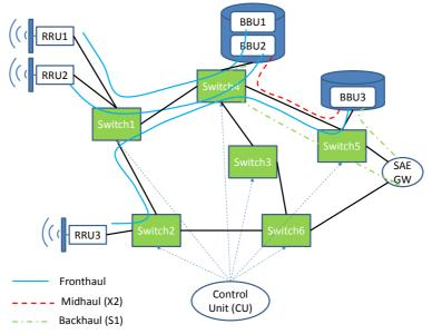
Figure 2 – Possible Xhaul network architecture
