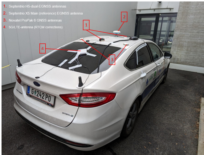
Figure 1. Automated Driving Demonstrator (ADD) vehicle antenna configuration during the path following experiments.
