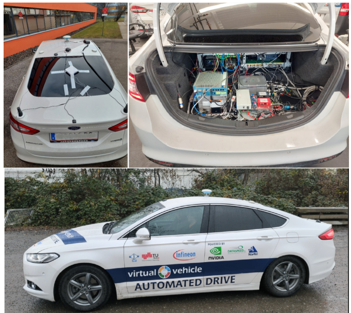
Figure 2. Automated Driving Demonstrator (ADD) vehicle based on the Ford Mondeo 2016 platform and DataSpeed drive-by-wire interface. The ADD vehicle is equipped with rudimentary EGNSS receiver/antenna configurations to analyse the effect of OSNMA on tracking performance.
