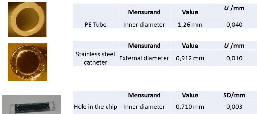
Figure 25: Dimensions measured using the interferometer for the PDMS chip; the assembly is shown in Figure 15.
