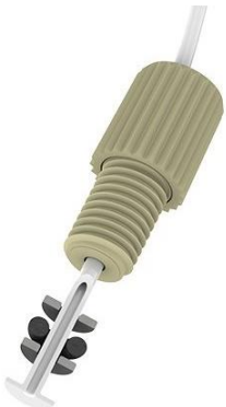
Figure 4: Flared fitting connection. The configurations of flared tubing assemblies are 1/16 - 1/8" OD plastic tubing such as PTFE, FEP, LDPE, or PEEK and with connections to 1/4-28, 10-32, M6, and 6-40 threaded ports.
