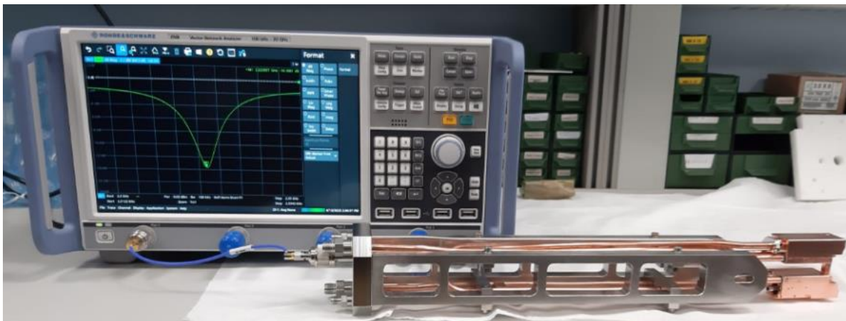
Figure 6.1. Ion source low power test configuration
