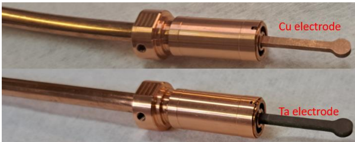
Figure 6.2. Copper and tantalum electrodes assembled on the ion source internal body
