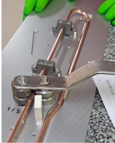
Figure 4.2: Bending step of a water-cooling tube
