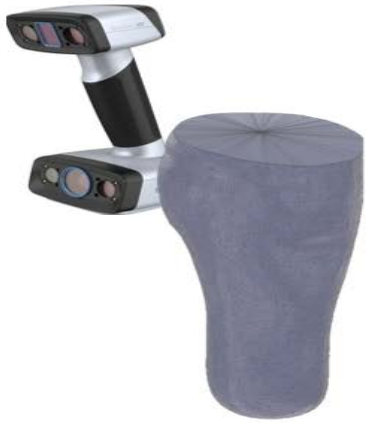
3D scanning of patient limb – point cloud data
