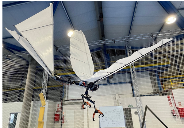
Fig. 1: The developed SMA actuated hip joint integrated on E-Flap ornithopter [8].
