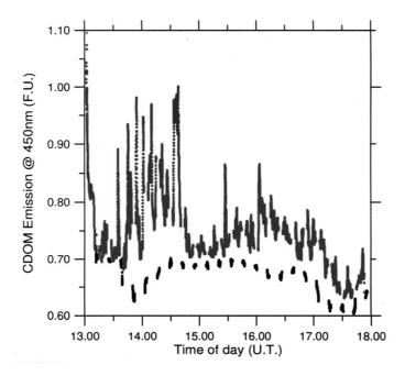
*Figure 3: Data obtained on Julian Day 130 from the NSF CoOP cruise of April/May 1995 aboard the R/V New Horizon. Results are from the time period between 13:00 to 18:00 Universal Time. The enhanced surface enrichment observed during the period between 13:30 and 14:30 correspond to a transit across a visibly slicked area.*
