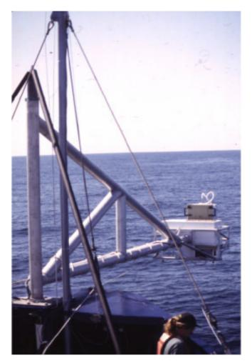
*Figure 2: The Controlled Heat Flux boom on the R/V New Horizon during the April/May 1995 NSF CoOP cruise off Monterey Bay.*
