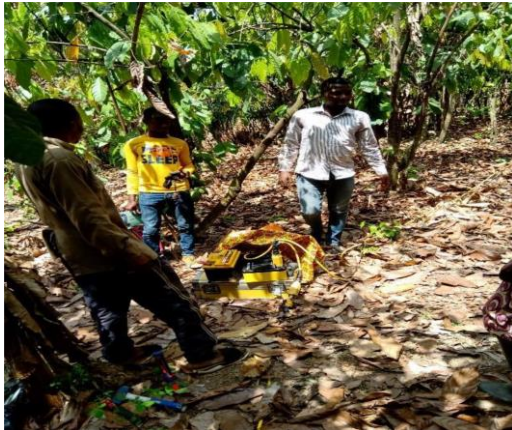
Figure 2a: Geophysical Crew Deploying ERT meter
