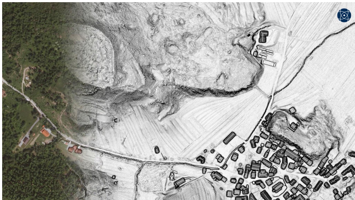
Figure 4. “Baba” Iron Age hillfort near Pivka Slovenia. Visualisation of airborne LiDAR data after the “removal” of vegetation, symbolized in the figure by aerial photography.
