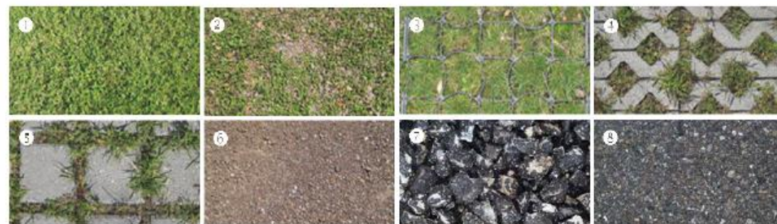
Figure 12: Overview of most common surfaces, from most to less permeable (source: Prokop et al., 2011).
