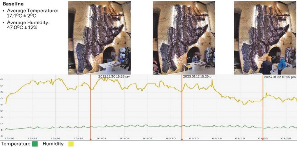
algorithms for data collection and analysis. The collected data show that the overall assembly had a negligible amount of shrinkage over the tracked period, which we can correlate to the observed stable temperature and humidity conditions in the exhibition space.
