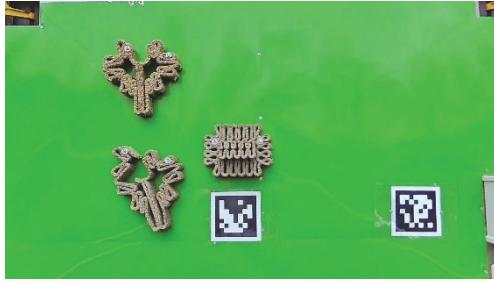
absorption from rain and humidity leads to expansion, while evaporation caused by solar radiation and high temperatures lead to contraction. The collected data showed that the collagen-based recipe has a stronger behaviour, where it transitions from a brittle condition to a flexible one as it absorbs moisture, and a reversed conditions as it dries. The xanthan gum-based recipe has also hygroscopic behaviour, in comparison it is though more stable.
