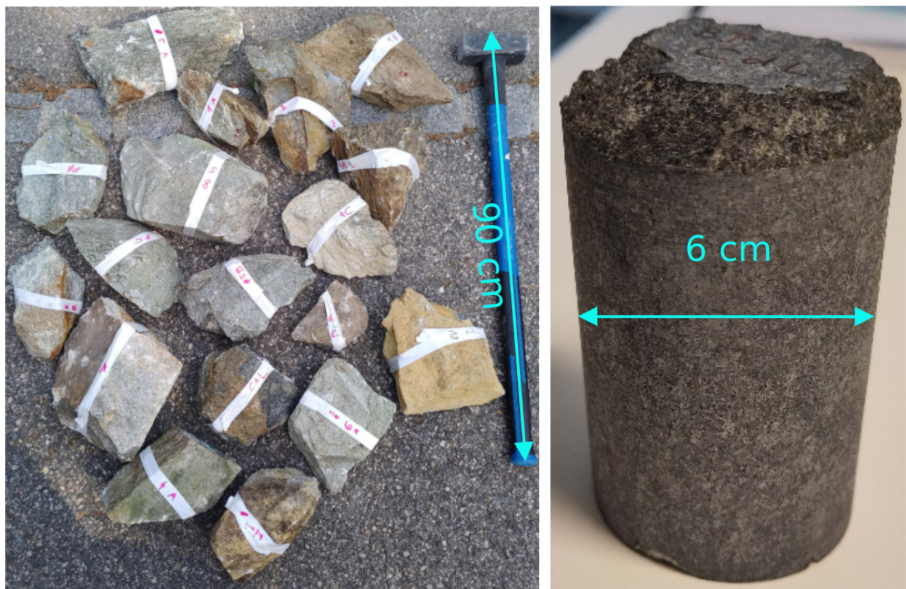
Figure 3. (a) Photo of the newly collected, larger rock samples before laboratory work. (b) One of the cut cylinders ready for Archimedes type density determination.
