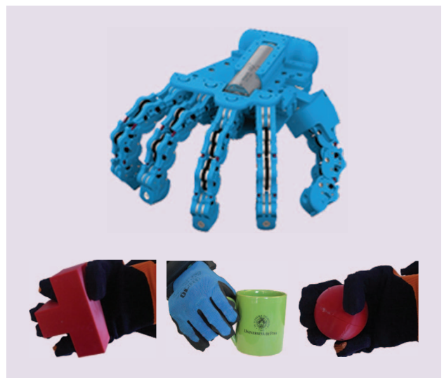
Figure 4. The Pisa/IIT SoftHand, a simple and robust robotic hand with 19 DoF but actuated by only one motor. Its closing movement replicates the synergy of the human hand.
