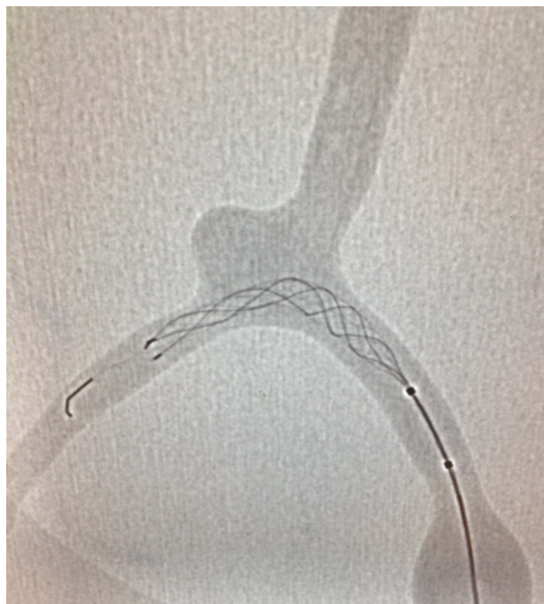
Figure 7. Silicone simulator with partially deployed LVIS Jr stent prior to applying forward tension to barrel the stent across aneurysm neck.
