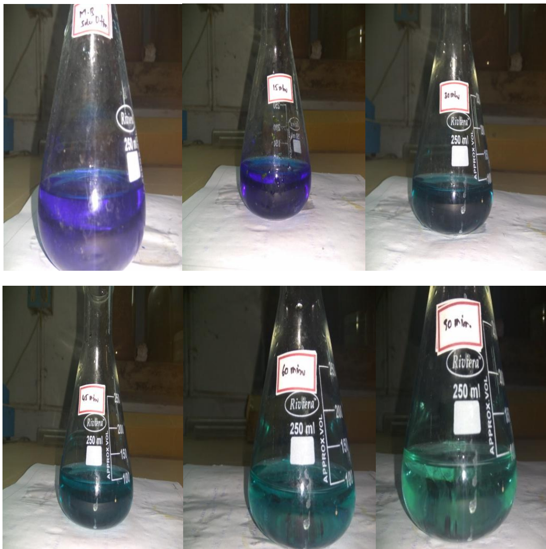
Fig.6: Colour change of methylene blue dye after addition of CuNPs.
