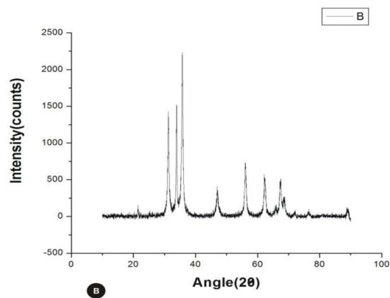
Fig-4: XRD analysis of ZnO-NPs of root extract of *R. Cordifolia*.
