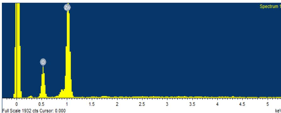
Fig-3: EDX measurement of ZnO-NPs of root extract of *R Cordifolia*.
