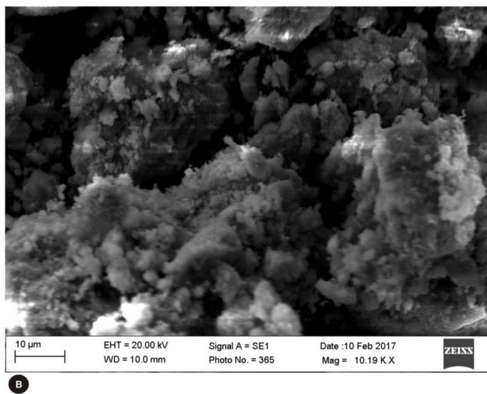
Fig-1: SEM analysis of ZnO-NPs of root extract of *R. Cordifolia*.
