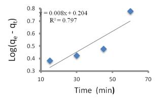
Figure 6 Pseudo-first-order kinetics plots for the adsorption of fluoride onto FC.
