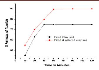
Figure 2: Effect of contact time on the adsorption of fluoride onto FC and FC-TLA (Initial concentration of fluoride ion =30 mg/L, adsorbent dose = 2 g, pH= 7 agitation speed = 150 rpm and temperature =  $25 \pm 2 \circ C$ ).
