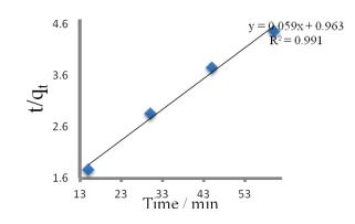
Figure 9 Pseudo-second-order kinetic plots for the adsorption of fluoride onto FC-TLA.
