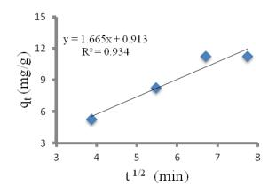
Figure 10 Intra particle diffusion curve for adsorption of fluoride onto FC at  $25 \pm 2$  °C temperature.
