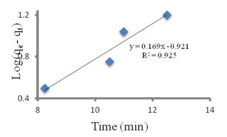
Figure 7 Pseudo-first-order kinetics plots for the adsorption of fluoride onto FC-TLA
