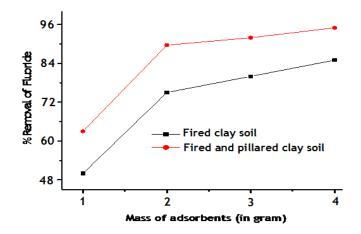
Figure 3: Effect of adsorbent dose on adsorption of fluoride onto FC and FC-TLA (Initial concentration of fluoride ion =30 mg/L, pH=7 contact time 45 min for FC, 60 min for FC-TLA, agitation speed = 150 rpm and temperature of  $25 \pm 2^{\circ}$ C).
