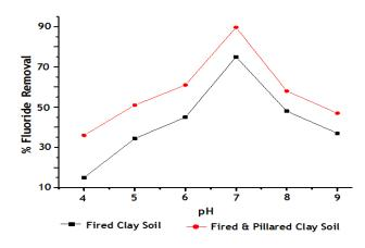
Figure 1: Effect of pH on adsorption of fluoride by FC and FC-TLA (Initial concentration of fluoride ion =30 mg/L, adsorbent dose = 2 g, contact time =120 min, agitation speed = 150 rpm and temperature =  $25 \pm 2^{\circ}$ C).
