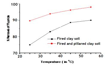
Figure 5: Effect of temperature on adsorption of fluoride onto FC and FC-TLA (Initial concentration of fluoride ion =30 mg/L, pH= 7, contact time 45 min for FC and 60 min for FC-TLA and adsorbent dose = 2 g and agitation speed = 150 rpm).
