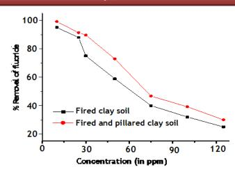
Figure 4: Effect of Initial fluoride ion concentration on adsorption efficiency of fluoride onto FC and FC-TLA) (pH= 7 contact time = 45 min for FC, 60 min for FC-TLA, adsorbent dose = 2 g, agitation speed = 150 rpm and temperature  $25 \pm 2 \circ C$ ).
