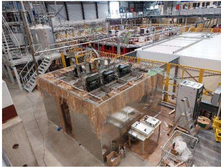
Fig. 3: CRP2 while being tested at warm in the Faraday cage setup before undergoing a cold-box test. The CRP is suspended from the cold-box roof which closes the top side of the Faraday Cage. The cold-box roof is fully instrumented with the analogue readout electronics and the uTCA digitization system and in a cold-box test in TPC mode.
