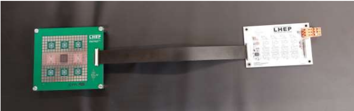
Figure 2: SiPM test board, Flex cable and the Pre-amplification board
