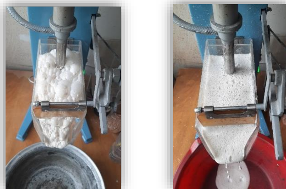
Figure 1. Dolomite mineral flotation process. a) enrichment process of dolomite with soapstock flotation agent. b) enrichment process of dolomite with UGK flotation agent.
