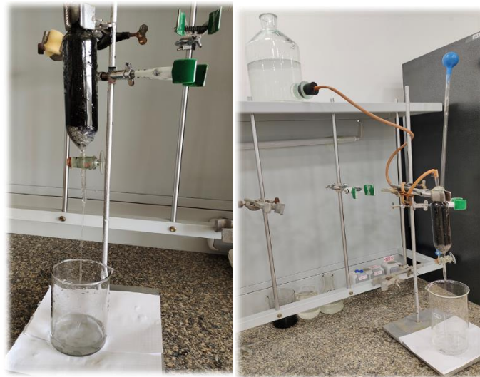
Figure 2. The process of washing bentonite-coal sorbents and industrial waste water treatment with them
