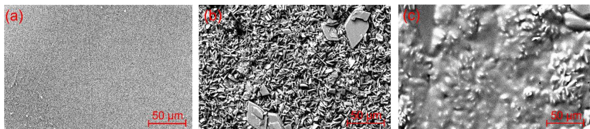
248 249 Fig. 3. SEM images of surface morphology of (a) PLA, (b) CaP, and (c) CaP-PLA coatings
