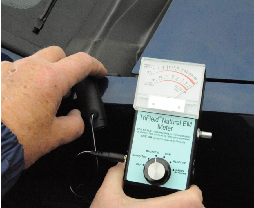
SUBJECT VEHICLE - Passenger's side (11-27-09) 36 hours after event rear engine compartment magnetic field reading. (Full intensity needle pegged)
