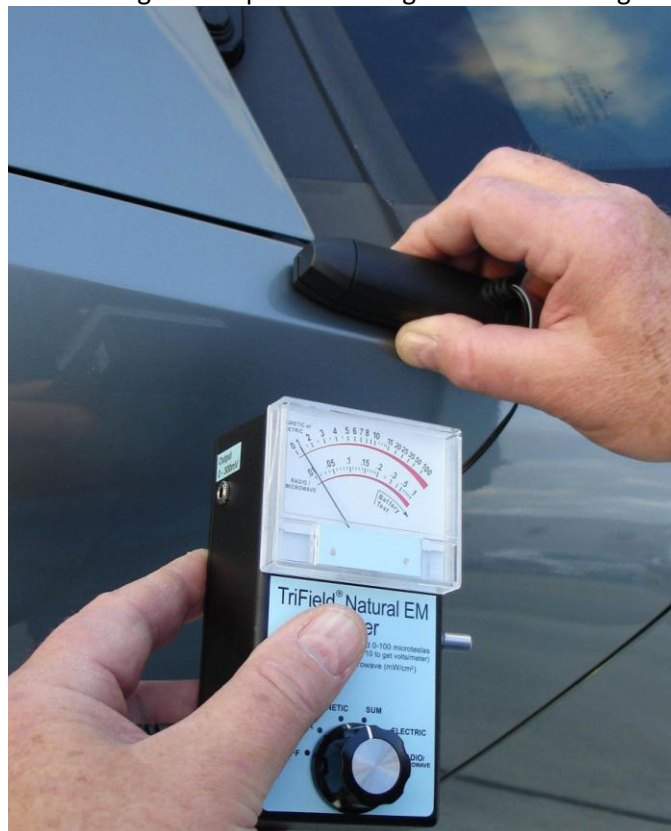
TEST VEHICLE - Driver's side rear engine compartment magnetic field reading.
