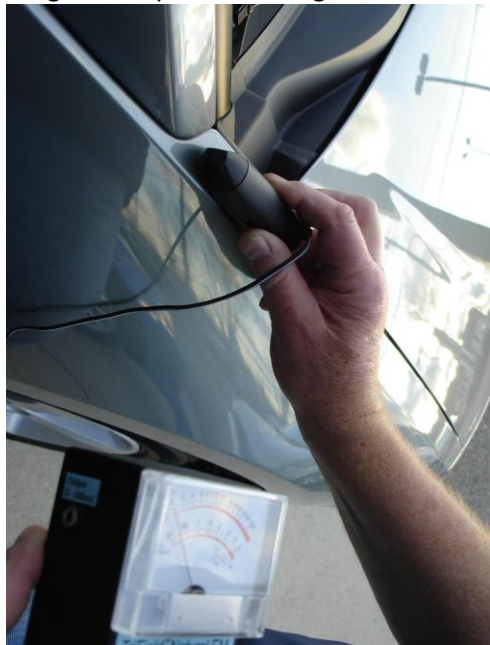
TEST VEHICLE - Passenger's side rear engine compartment magnetic field reading
