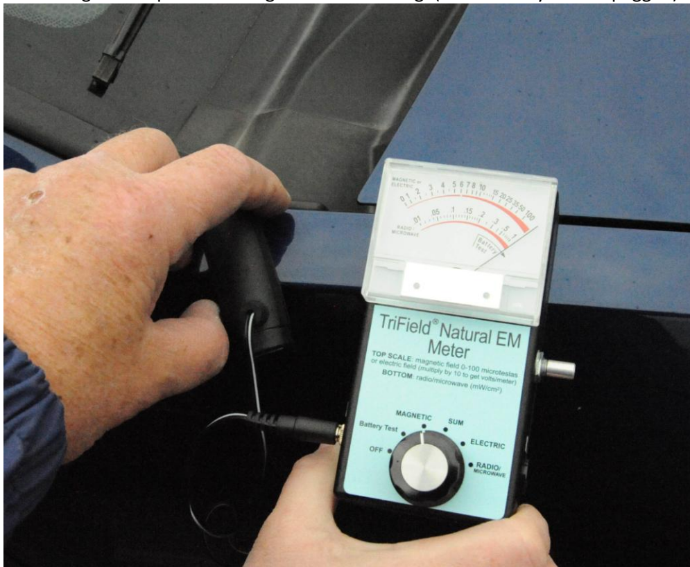
SUBJECT VEHICLE - Passenger's side rear engine compartment magnetic field reading. (Full intensity needle pegged)
