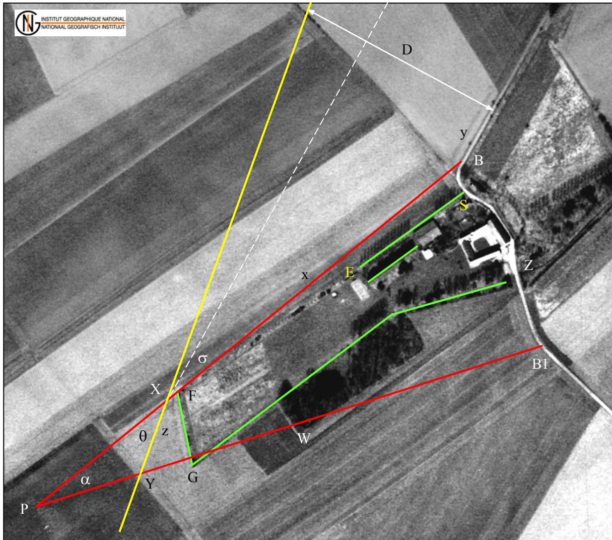
Figure 16: Aerial picture of 1995 (© NGI ) with the critical lines of sight at B and B1, a fraction of the trajectory (in yellow) and the rows of high poplars that were present in December 1989 (in green).
