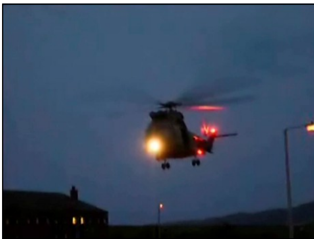
Figure 22: Landing lights of a SAE-330 Puma.
