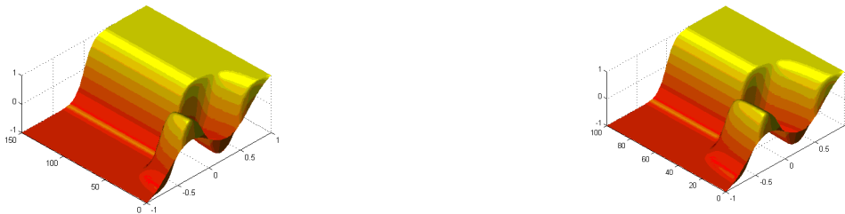
Fig.2. Time evolution for the Allen-Kahn equation N=120 and \varepsilon = 0.01 . The x-axis runs from x=-1 to x=1 and the t-axis runs from t=150 to t=200 s.
