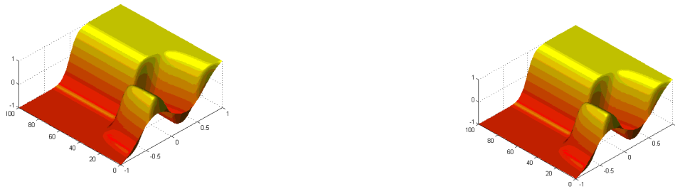
Fig.1. Time evolution for the Allen-Kahn equation N=120 and \varepsilon = 0.01 . The x-axis runs from x=-1 to x=1 and the t-axis runs from t=0 to t=150 s.
