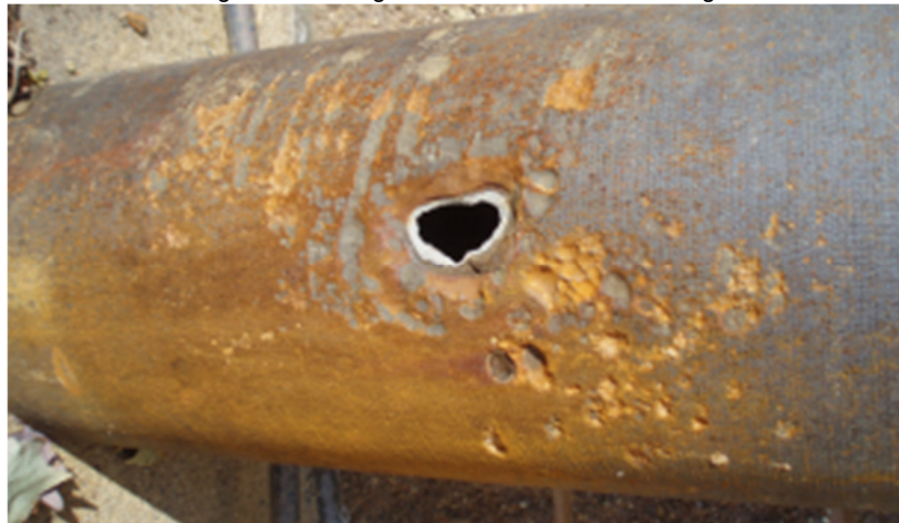
Figure 5-7. External pitting corrosion in underground pipe
