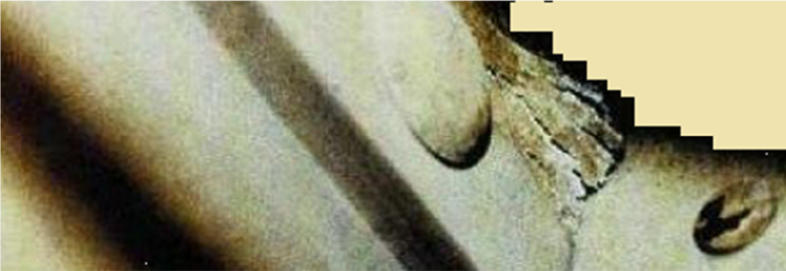
Fig. 5- 52. Exfoliation of aluminum.
