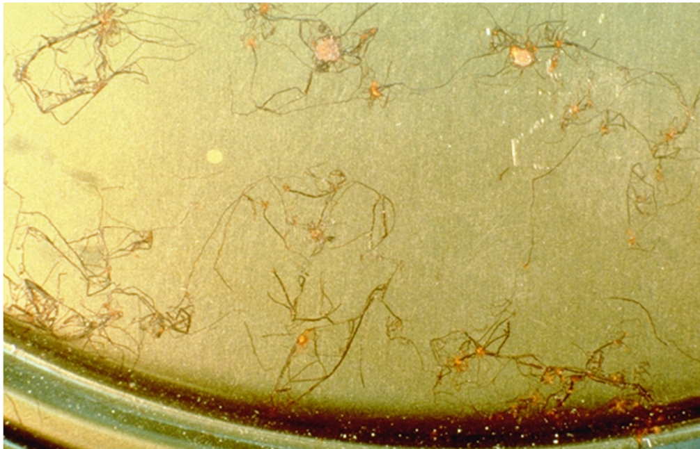
Fig. 5-16. Filiform corrosion on steel drum lid
