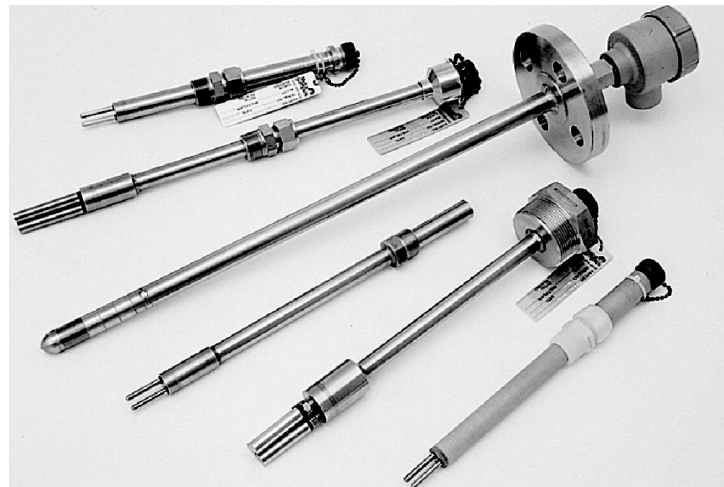
Fig. 8-11. Commercial sensor elements to carry out linear polarization resistance (LPR) measurements.
