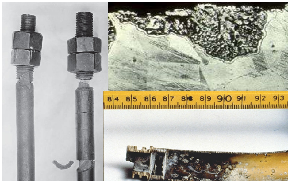
Fig. 5- 53. Left Layer-type dezincification in brass bolts. The brass on the top right dezincified leaving a porous copper plug on the surface. Right bottom: dezincification of Mixing Tap Orifice - Potable Water.
