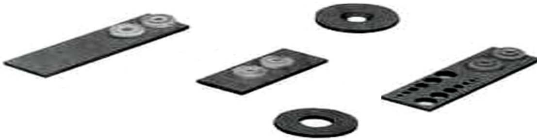
Fig. 8-2. Corrosion coupon types.
