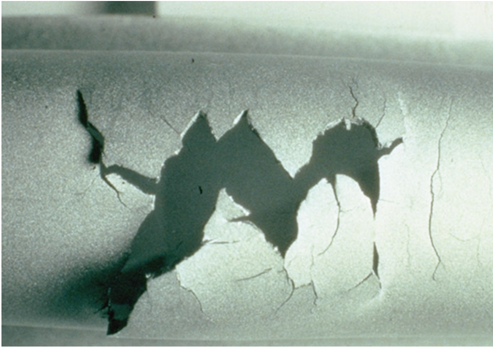
Fig. 5-30. SCC on Stainless Steel Expansion Joint - Alkaline Water in Steam Line.
