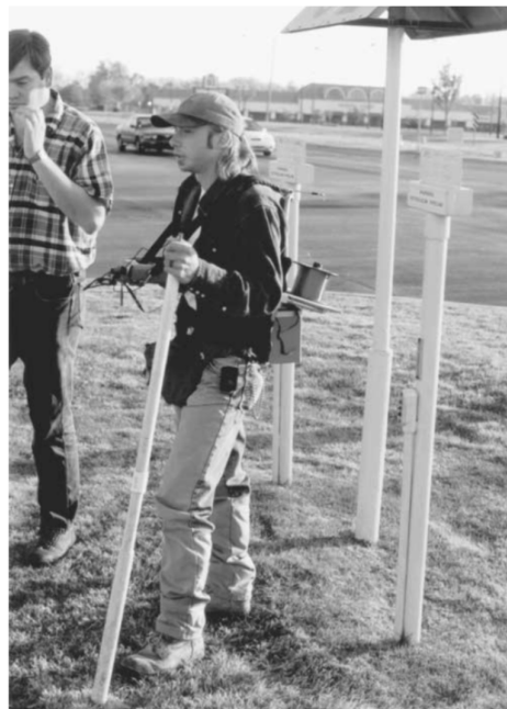
Figure 9.22 CIPS equipment, with the operator starting a survey at a test post.
