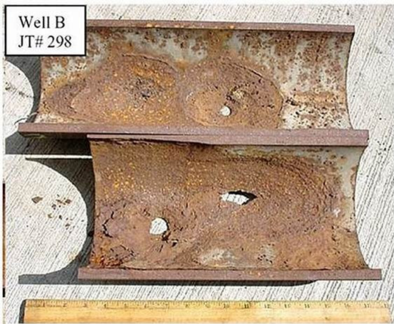
Figure 5-7. External pitting corrosion in underground pipe
