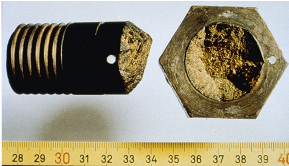
Fig 5-34. SCC of Aluminum Brass Bolt - Steam with Traces of Ammonia.
