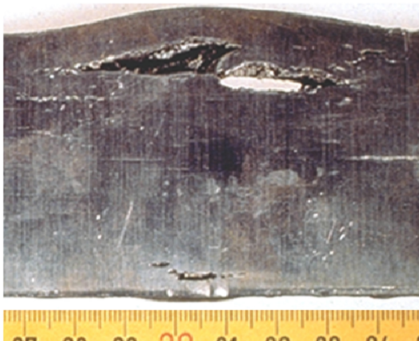
Fig 5-37. Hot Hydrogen Attack of Carbon Steel Plate - Naphtha + Hydrogen at 500 C
