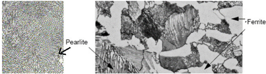
Fig. A-2. Pearlite (left) – Ferrite and pearlite (right).
