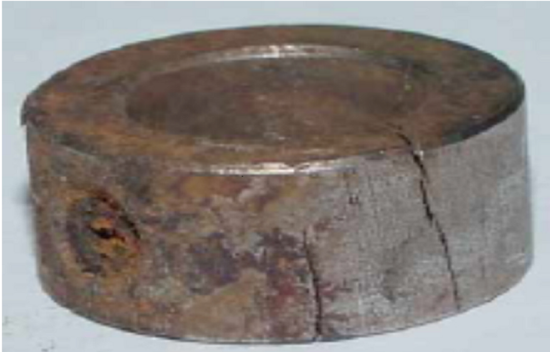
Fig. 5-32. Chloride induced stress corrosion cracking
