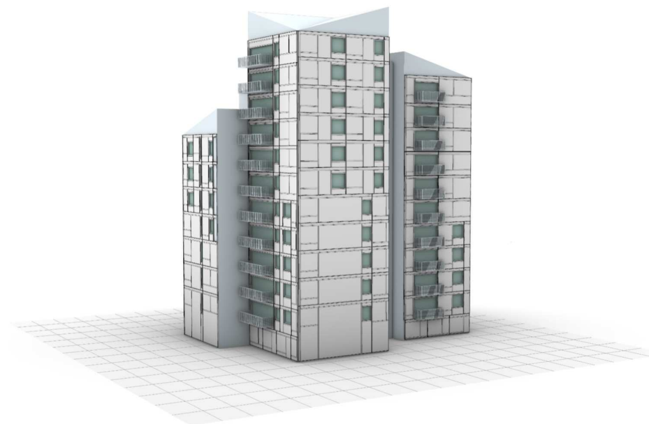
Figure 10. Output of the code described in this section RG1.2, that includes prefabricated layout definition including solar panels and registration areas in the building model of demo-building in Milan, Italy.
