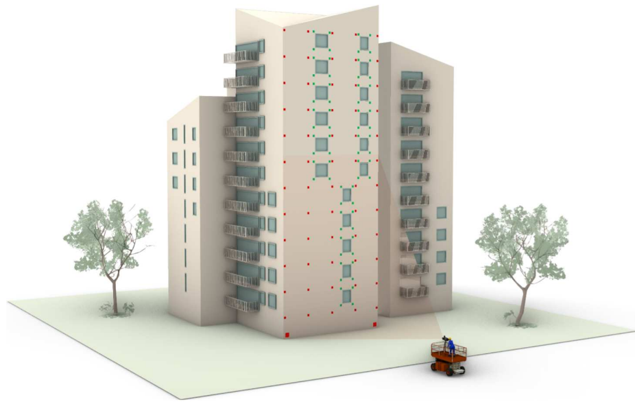
Figure 11. Capturing the real building images with AprilTags, which are located in the critical points of the facade. Example of the demo building in Milan.
