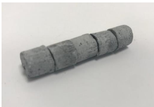
Figure 1. Waterjet cut ENG discs after impregnation with salt and drying.
