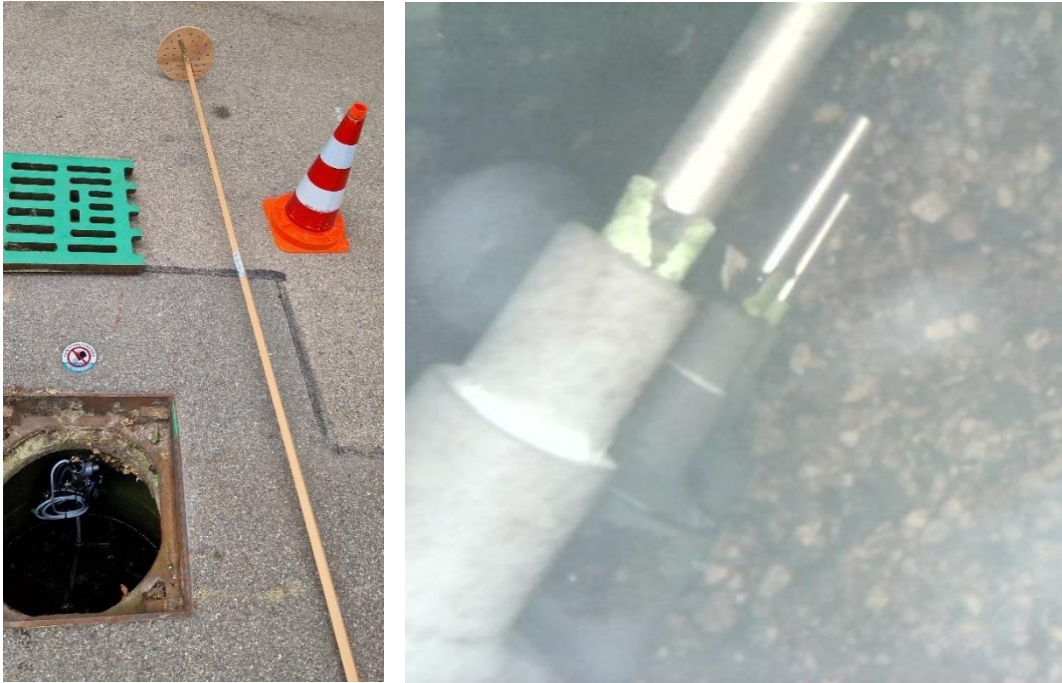
Figure 4: Sediment depth measurement tool (left) and endoscope photo (right).
