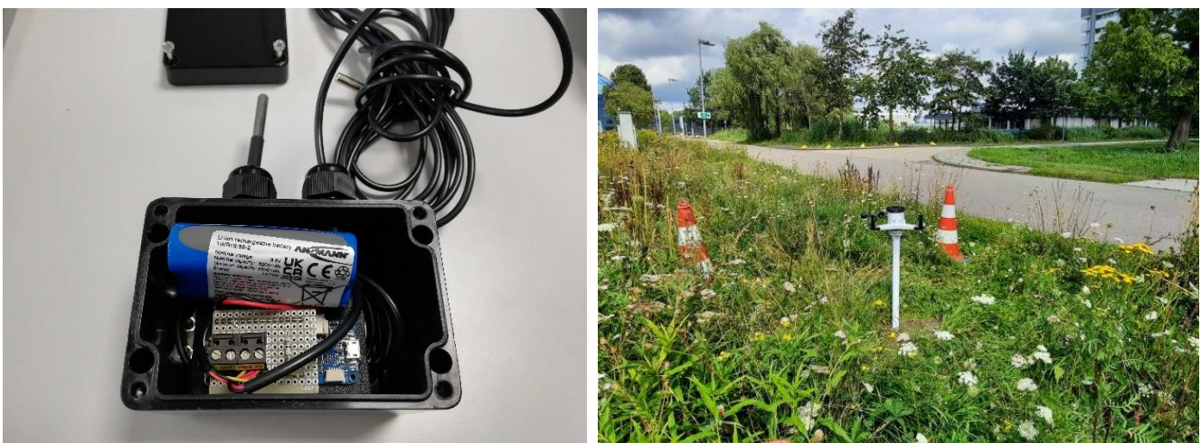
Figure 3. First version for measuring temperature dynamics in real gully pots (left) and weather station at Deltares Campus (right) (MetOffice, 2023).
