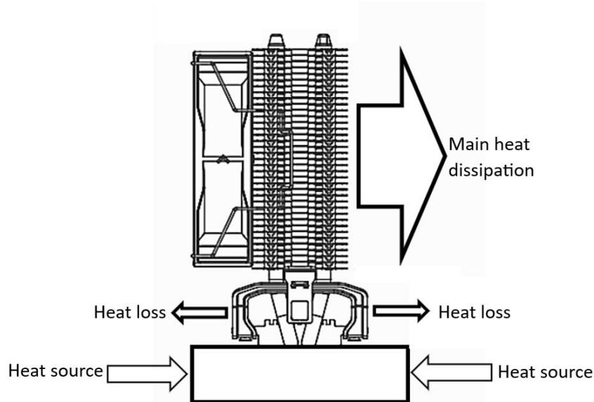
**FIGURE 1: Temperature flow through the experimental device**
