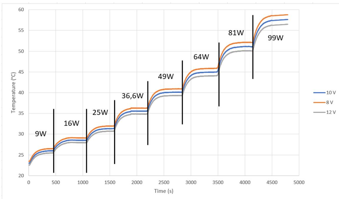
**FIGURE 4: Change in maximum temperature with different heat outputs of heating elements and fan speed over time**
