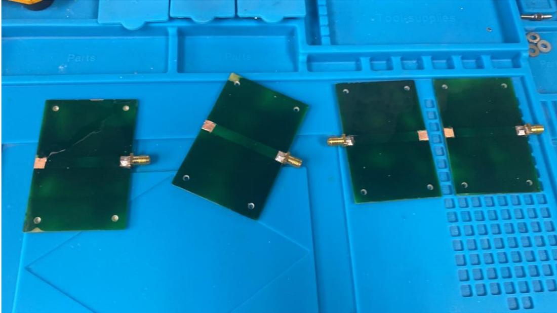
**Fig. 8.** RF applicators superior sections
