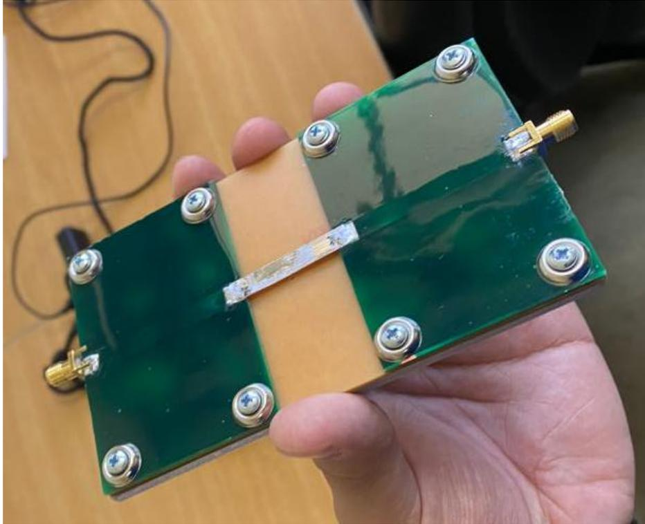
**Fig. 10.** RF applicator post-assembly
