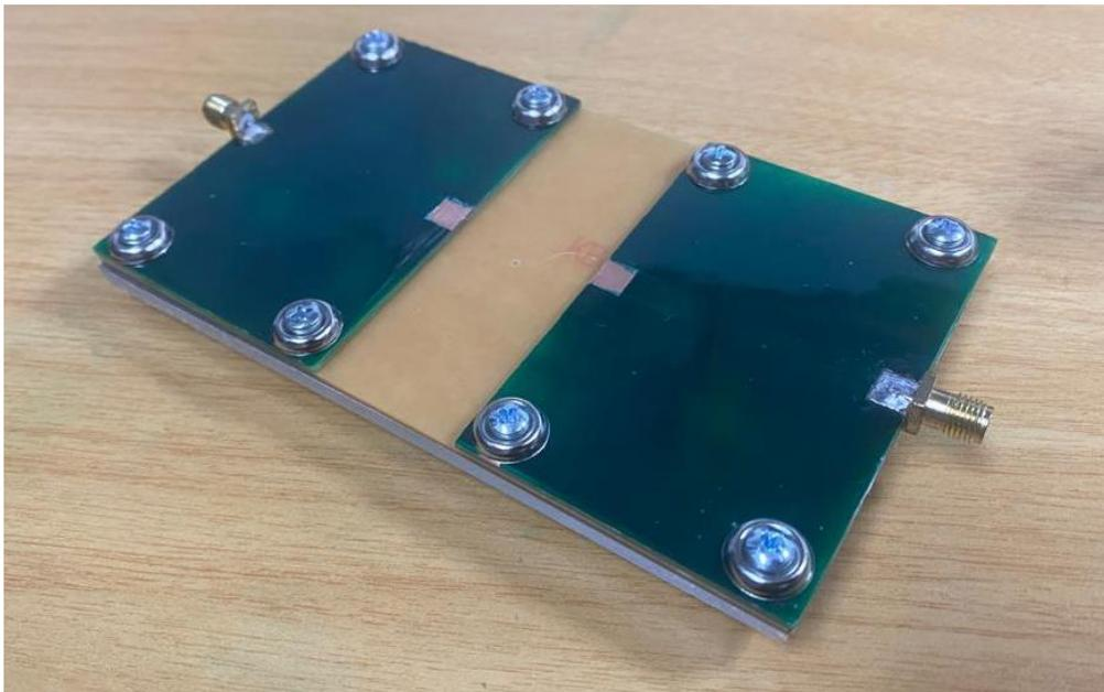
**Fig. 9.** RF applicator post-assembly
