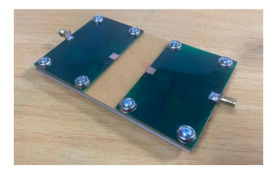
Fig. 9. RF applicator post-assembly
