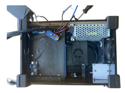
Fig. 4. Placement of the control circuit support part
