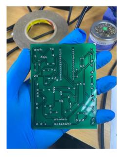
Fig. 5. Control circuit post – solder mask application
