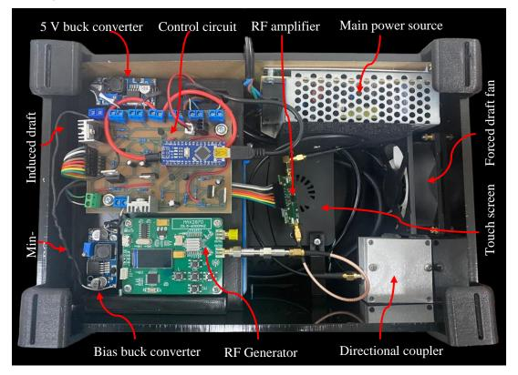
Fig. 6. Internal composition of the irradiation prototype
