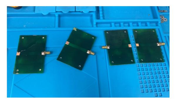
Fig. 8. RF applicators superior sections
