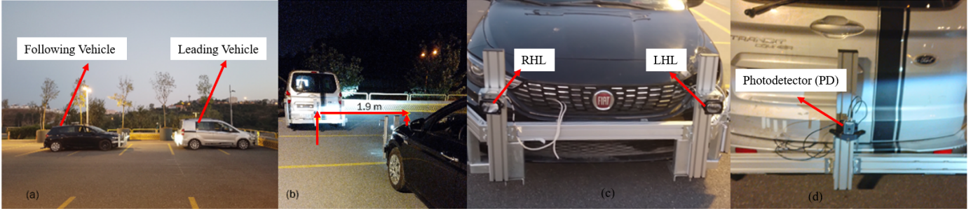
Fig. 4: (a) Both vehicles aligned (b) 1.9 m lateral shift between both vehicles (c) Both LHL and RHL attached to following vehicle at a height of 70 cm from ground and (d) PD attached to leading vehicle at a height of 60 cm from ground.
