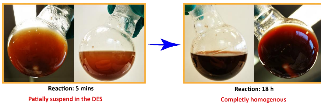
Figure S1. Pictures of the reaction at initial 5 mins and 18. Reaction time: reaction condition: 12.6 g (90 mmol) ChCl, 10.8 g (180 mmol) EG, 500 mg REL from walnut shell, 2.11 g oxalic acid (9%, based on the total mass of ChCl and EG) at 80°C for 18 h.
