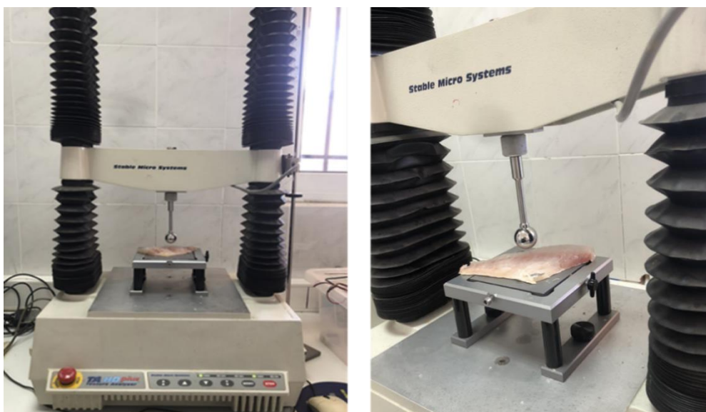
Figure 55 Analysis of seabream fillets using a HD-Plus texture analyzer (Stable Micro Pedicels Ltd., Godalming, UK)
