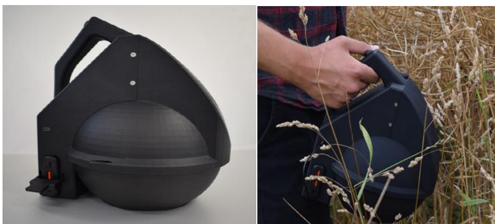
Figure 58. VideometerLite, portable handheld multispectral imaging device.
