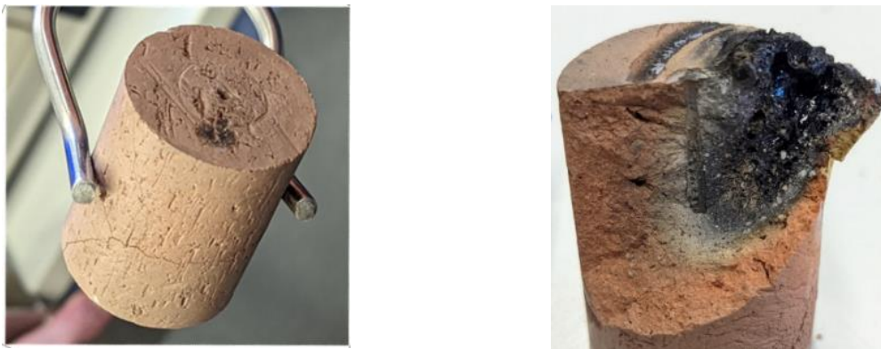
Fig. 1. Pictures of thermal runaway in specimen with microwave-assisted firing. On the left with local discolouration and on the right with swelling and vitrification.
