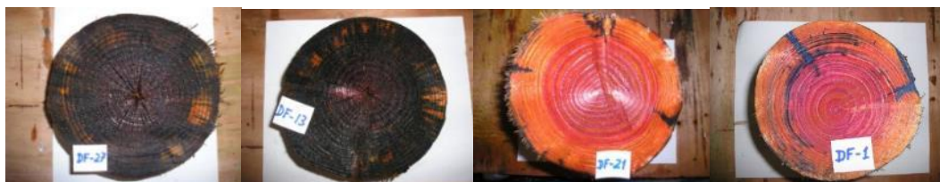
Fig. 4. Solution distribution in Douglas fir log cross section after MW modification and impregnation (left photos) and controls (right photos).
