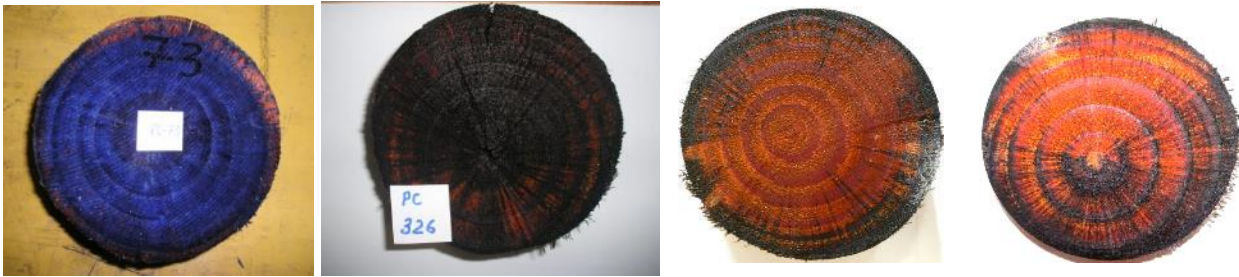
Fig. 5. Solution distribution in Radiata peeler core cross section after MW modification and impregnation (left photos) and controls (right photos).
