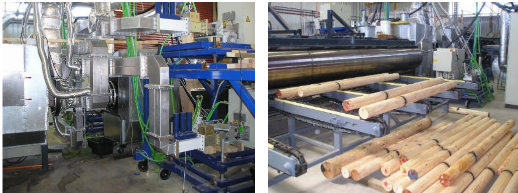
Fig. 2. 300 kW MW experimental Plant for timber modification.
