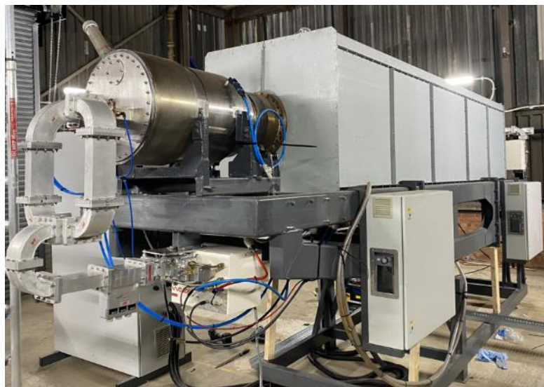
Fig. 2. Pilot Scale Microwave hybrid rotary kiln for reduction of iron ore.
