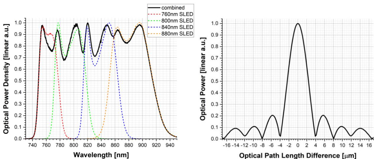
Fig. 2 Left: Optical spectrum of individual SLEDs (dashed line) and of combined source (solid line); Right: Coherence function of combined-SLED source with a coherence length of 2.4  $\mu\text{m}$  (in air).
