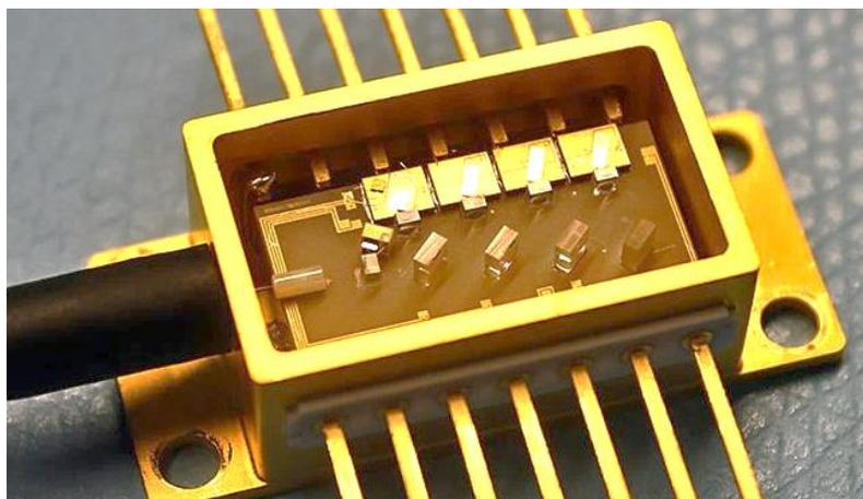
*Fig. 1: Photograph of combined-SLED broadband light source in 14-pin Butterfly module*
