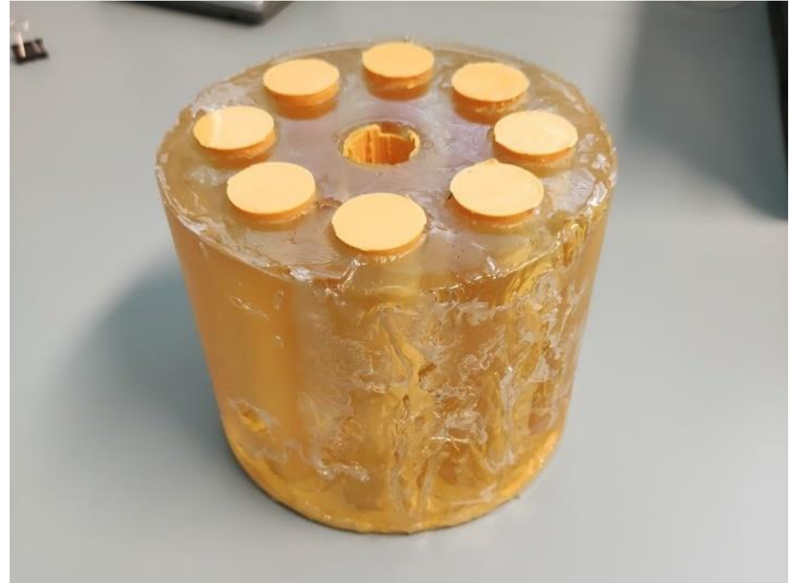
Bonus photo! Sad attempt to make a phantom using a plant pot, 3D printed negative plugs, and poured epoxy resin.
