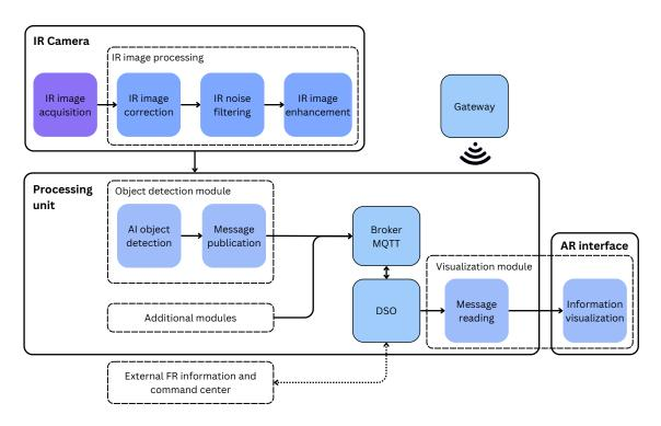
FIGURE 1. General architecture of the Smart Helmet. It is mainly divided into three devices interconnected between them, which are the IR camera, the processing unit, and the AR interface. Each of these components present inside the main operational modules that participate in the Smart helmet functions.
