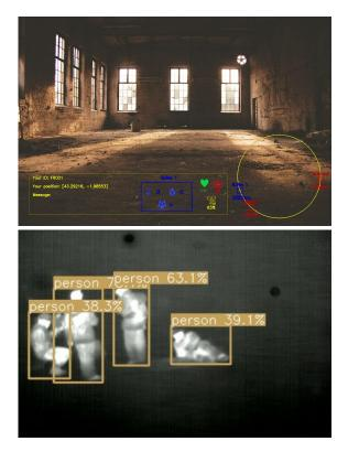
**FIGURE 4.** Examples of the smart visualization displayed on HUD. The upper part represents the visualization of the combined information on top of reality. The lower part shows the visualization of the thermal video stream with an object detection algorithm running on top, where 4 people are detected.
