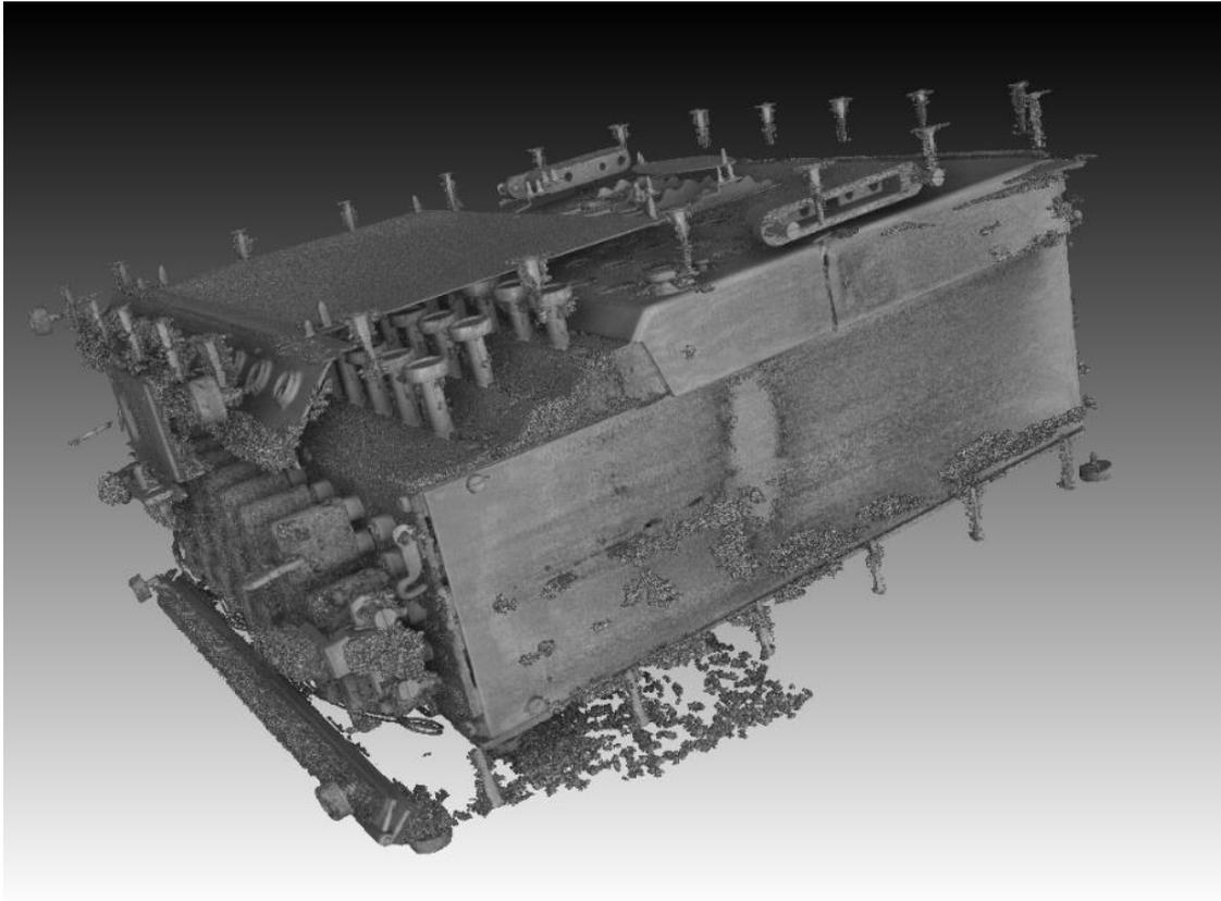
Figure 5. Unclean surface determination of an Enigma M4 with artefacts.
