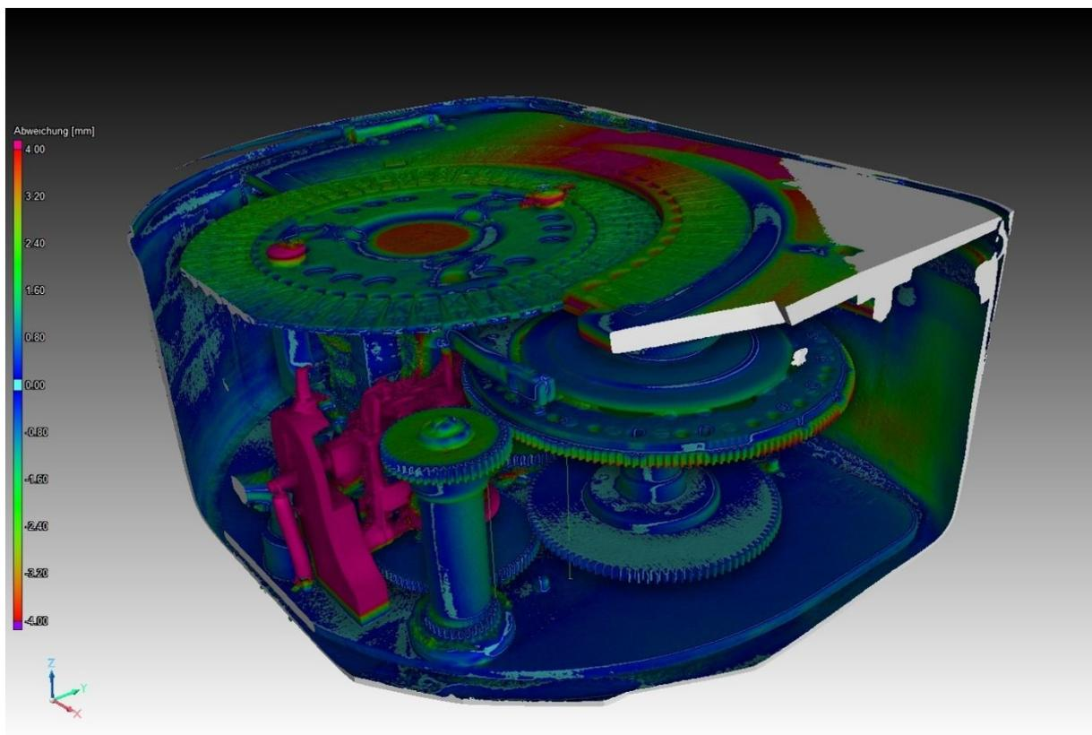
Figure 8. Digital overlay of two Kryha standard machines with coloured deviation diagram. The pink-coloured mechanics at the bottom left of the picture are not present in the comparison object.
