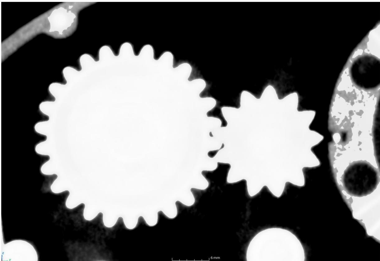
Figure 10. 2D-CT image of two apparently fused gears.
