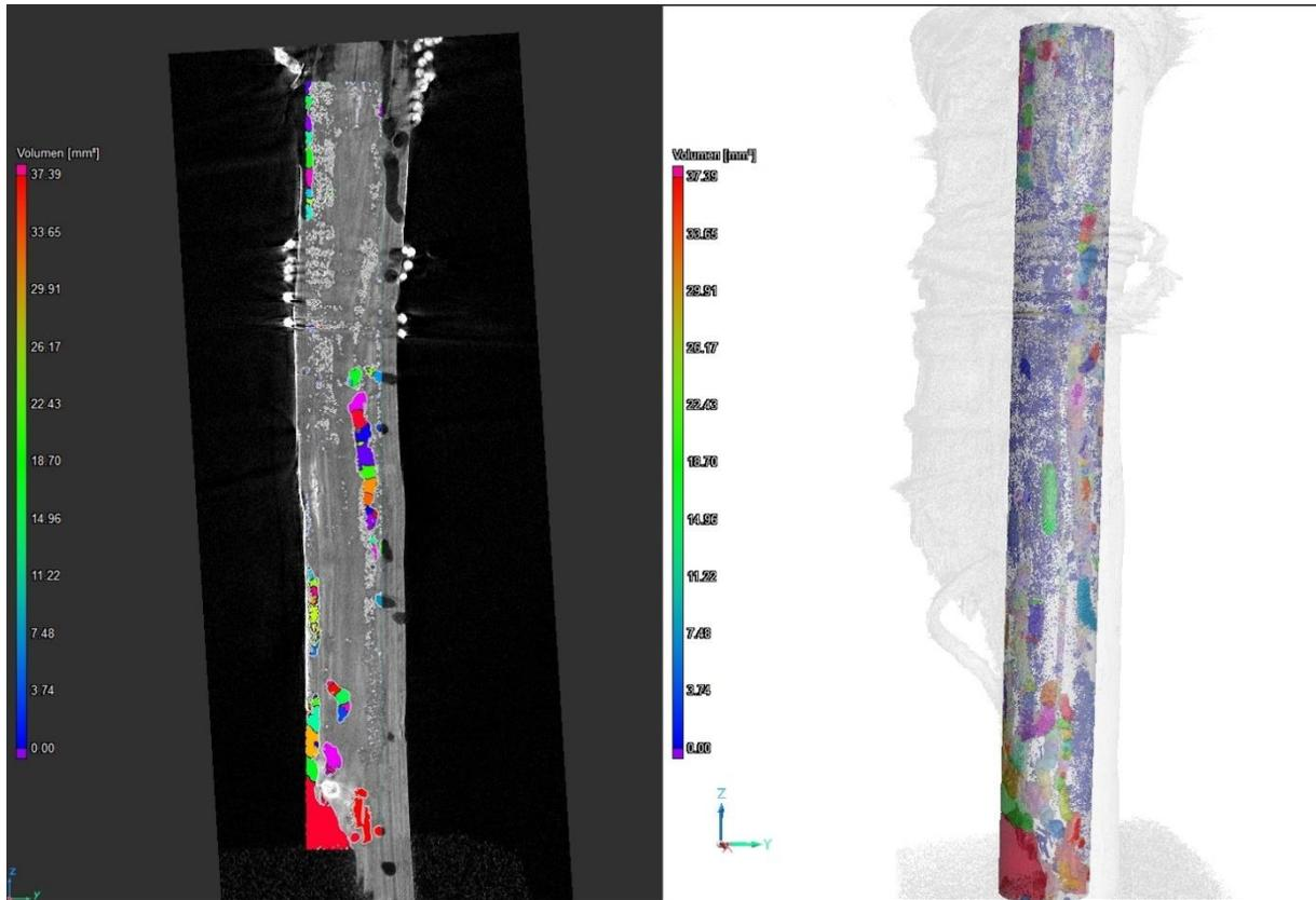
Figure 9. Porosity analysis of a strut of a glider by Otto Lilienthal in 2D and 3D view. The coloured areas depict air pockets that have been categorised and defined according to pore size.
