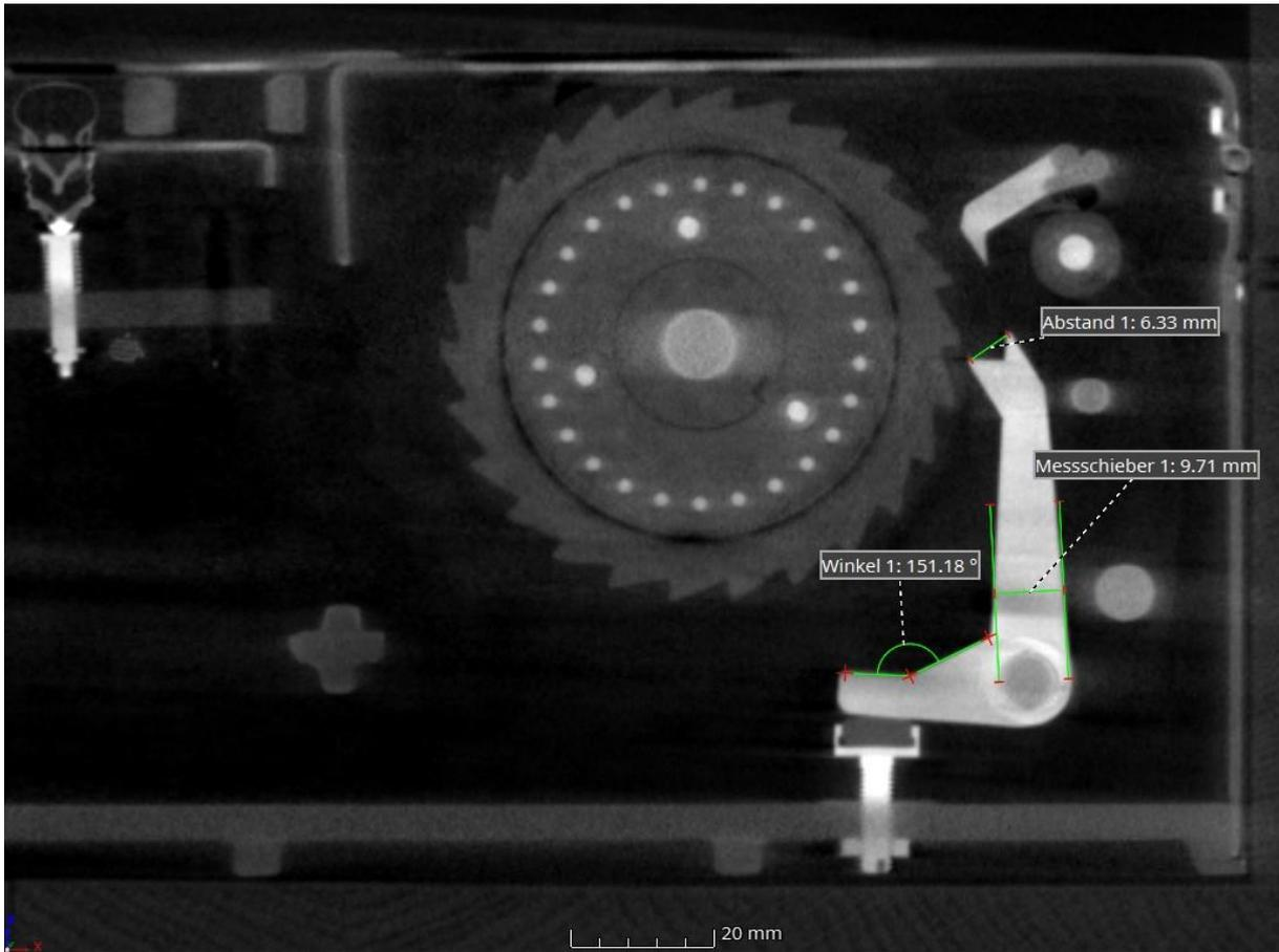
Figure 6. Distance and angle analyses on components of an Enigma M4.
