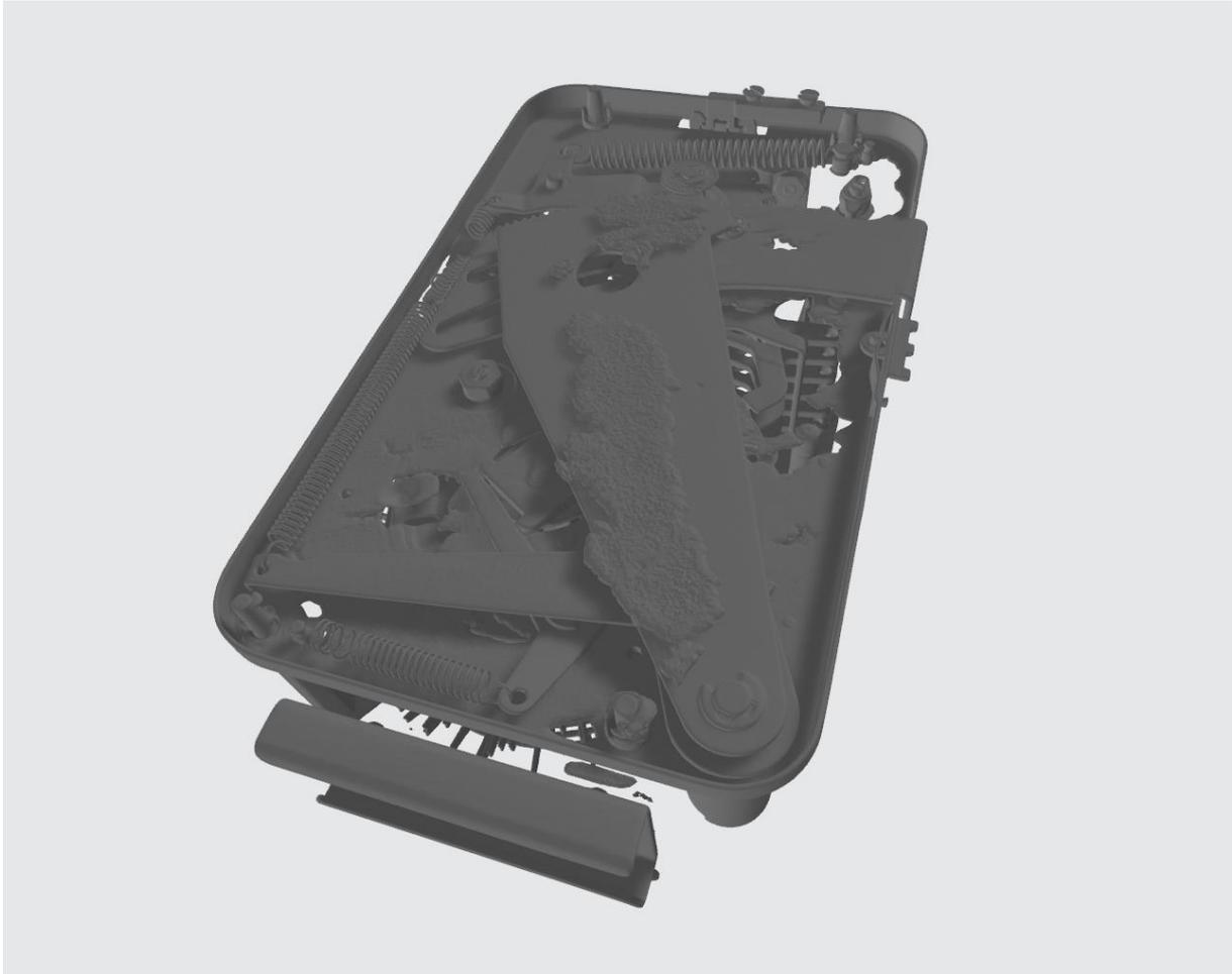
Figure 14. An unclean surface model with incorrectly recognised material as well as gaps due to unclean surface determination of the CT data. Hagelin CD-57 cipher machine.
