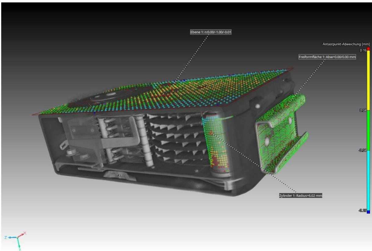
Figure 7. Geometric shapes adapted to a CT data set and the real deviations.
