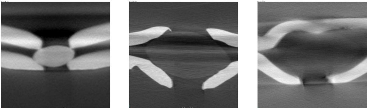
Figure 1. Differently pronounced beam hardening in three different single-lens microscopes. The lens in the left CT scan can be seen very well, while it can only be guessed at in the right image.
