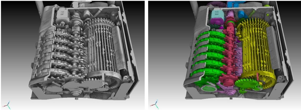
Figures 12 and 13. Unsegmented and segmented mechanics of the Hagelin M-209.
