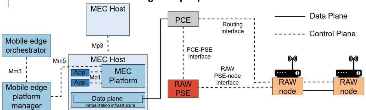
In the MEC reference architecture the Virtualisation infrastructure in the MEC host includes a **data plane that executes the traffic rules** received by the MEC platform, and routes the traffic among applications, services, DNS server/proxy, 3GPP network, **local networks and external networks**
