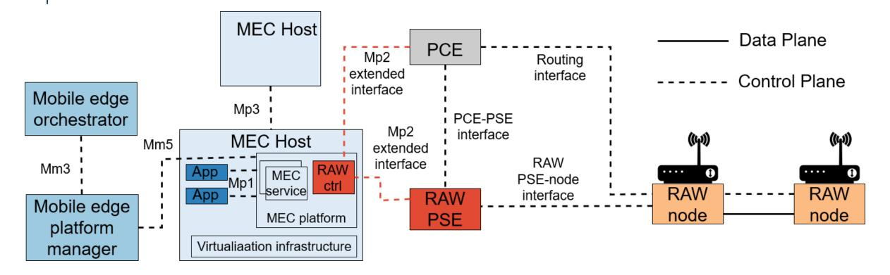
The Mp2 reference point between the MEC platform and the data plane of the Virtualisation infrastructure is used to instruct the data plane on how to route traffic among applications, networks, services, etc. **This reference point is not further specified.**
